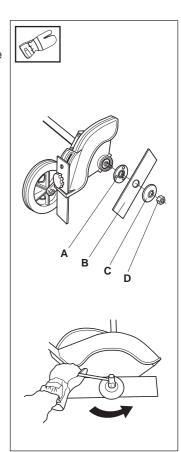
NOTE! Do not forget to remove the locking pin before using the machine.
